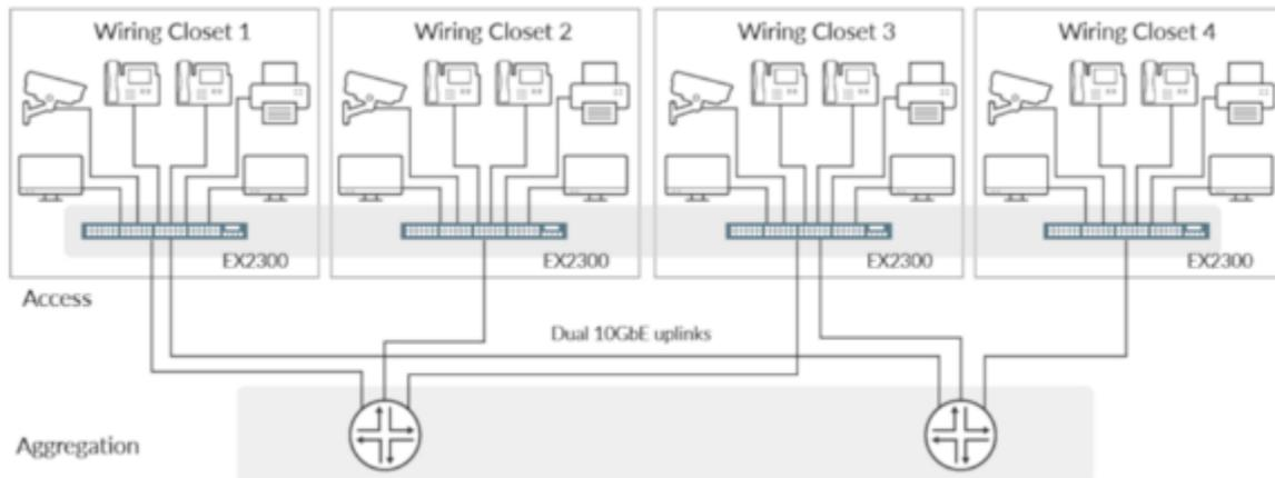
Figure 1: EX2300 switches support Virtual Chassis technology, which enables up to four interconnected switches to operate as a single, logical device.
